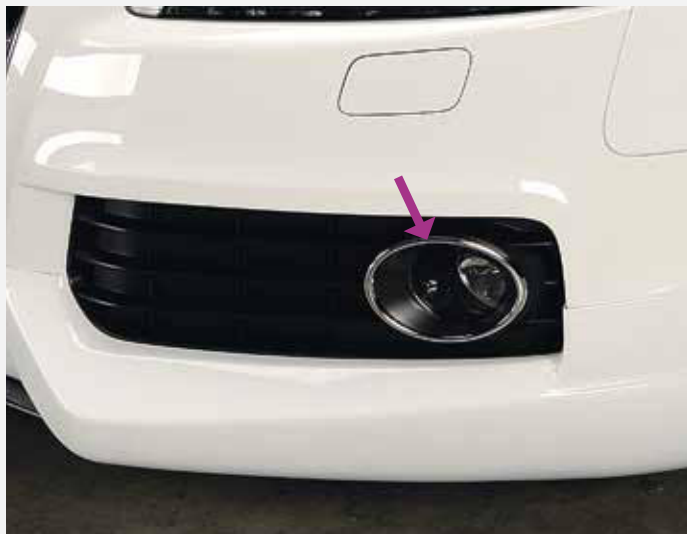
S-Line: fog lamp inside of the cover
