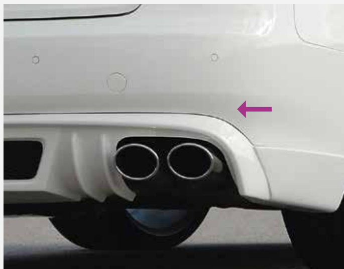
Not S-Line: no light edge above the rear skirt insert
