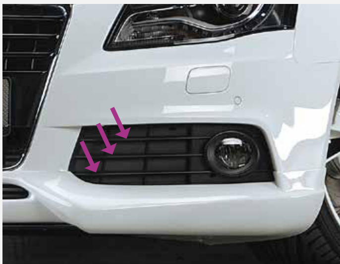
Not S-Line: three strips in the fog lamp cover
